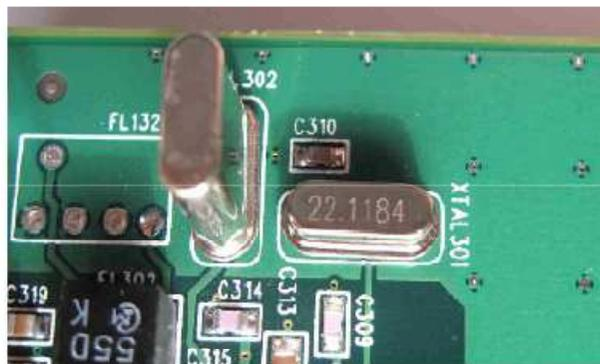
Figure 6.8. The second local oscillator; the quartz 22.1184 is in HC-49S format
