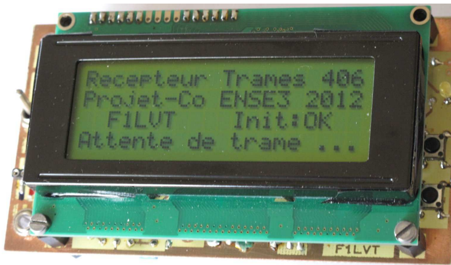
Photo 1: The frame decoder with the display of the homepage. Everything is ready for operation
