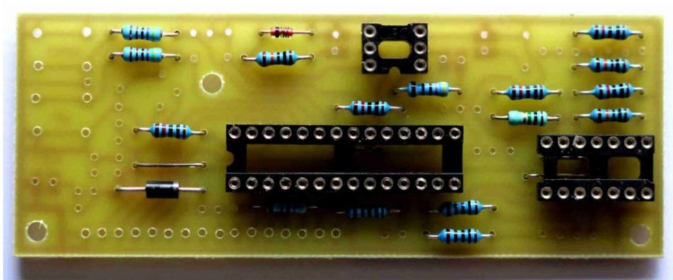
*Photo 3: The card with brackets and mounted resistors*
