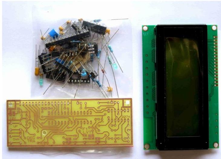
*Photo 1: All components for the decoder 406*
