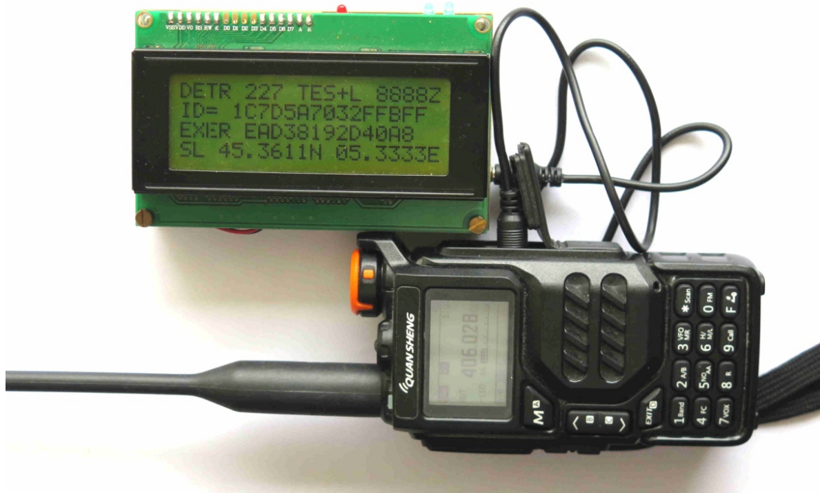
Photo 5: Operation of the "Quansheng UV-K5 + decoder" system
