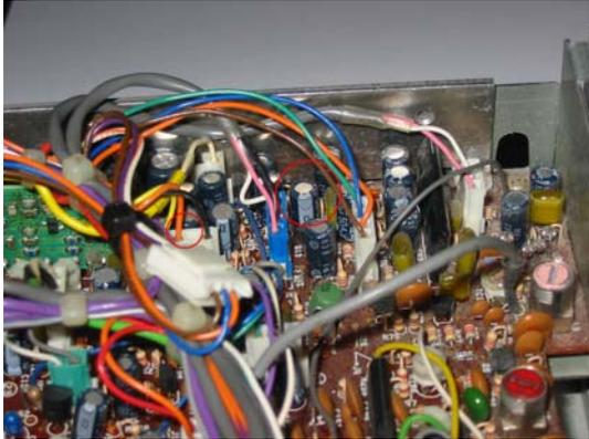
**Photo 2:** The corner of the board "IF Unit" as seen when the upper case is removed. You can see the C69 capacitor at the rear, behind C76, between the 2 connectors J2 (blue) and J6 (white), close to board edge. You can also see the J3 connector (white) with its orange wire connected to the +8V.
