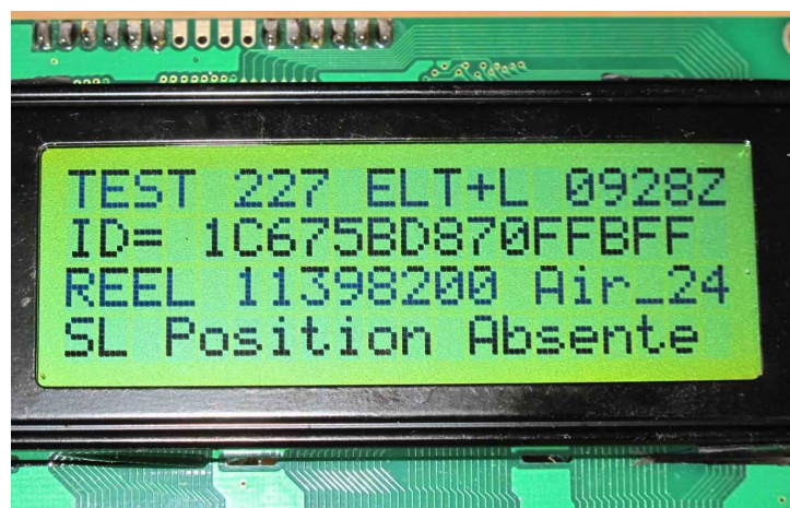
Photo 5 : Message transmitted by a beacon that should give its position, but the GPS of the beacon does not work. The time of reception is displayed.
