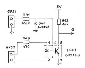
Figure 7: Schematic of the GPS input
