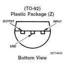
Figure 3: Pin assignment 78L05 5V 100mA regulator
