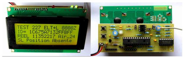
Photo 1 and 2: The frame decoder with its new DECTRA PCB and display. Above the display, you can see the lighted green LED 2 for monitoring system operation.
