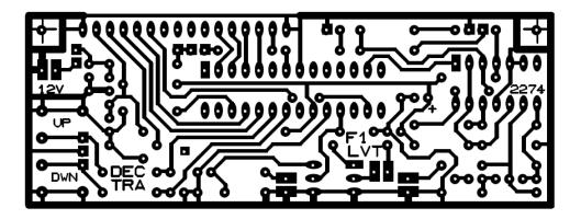
Figure 1: Printed Circuit DECTRA (trace side)
