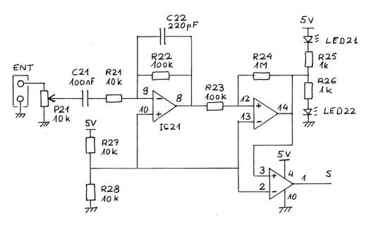
Figure 5: Diagram of input circuit
