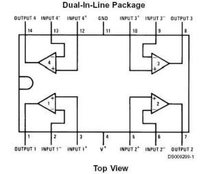
Figure 2: Pin assignment TLC2274 (classic pin for a quad op amp.)
