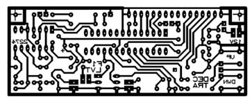
Figure 1: PCB component side seen at scale 1:1
