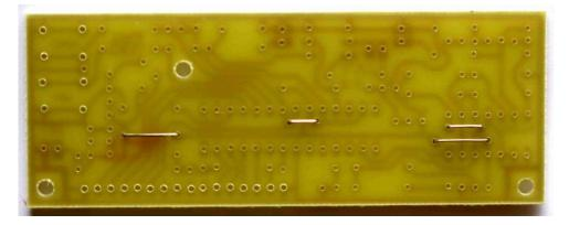
Photo 2: Installation of 4 jumpers
