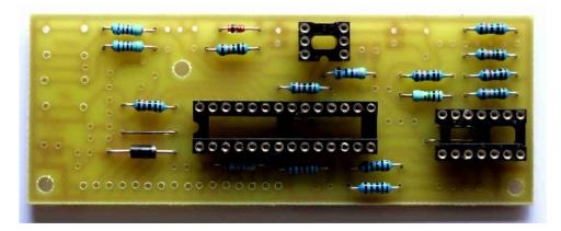
Photo 3: The card with brackets and mounted resistors
