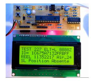
Photo 9: With the programmed PIC installed, the Home screen appears when power is applied
