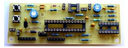
Photo 4 The card is almost finished, there remains the assembly of 3 LED side tracks.
