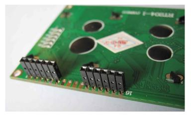
Photo 7: 2 female 6 pin connectors soldered under the display
