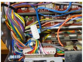
**Photo 9**: The connecting cable is plugged in the J54 connector behind the front face. This connector is not plugged any more in the "Control Unit" board; it is now connected only to the connecting cable with DSP module.
