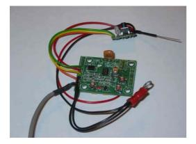
**Photo 1**: DSP module NEDSP1061-KBD from "bhi". The central part is connected to small command board, with a pushbutton and a LED. Connections are done by:
