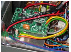
**Photo 10**: The two other wire ends are welded in parallel with the legs of the push-button of the command board of the DSP module. Attention to strictly respecting the colours because the pushbutton functions by ground connection of a positive tension.
