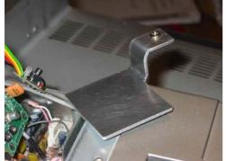
Photo 3: Manufacturing of the support to fix the DSP module. The flat part approximately measures 40 mm x 40 mm.
