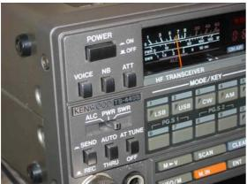
**Photo 6**: In the left higher angle of the TS440 front, near to the PB "Power" you find the PB "Voice". If option VS1 (Voice Synthesizer) is not inside, this push-button is available to control the DSP.
