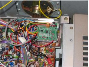
**Photo 4:** The support is fixed on the TX frame on a fixing point of the "IF Unit" board. The main board and the command board are fixed on the support with a two-part epoxy adhesive. The mass is screwed on a board fixation in bottom of the photo. The wire "+" is plugged in pin 2 of the connector J3 (orange wire with +8V in the white connector).
