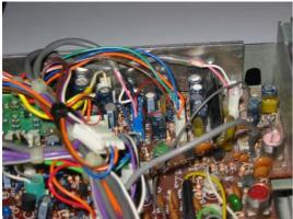
**Photo 2**: The corner of the board "IF Unit" as saw when the upper case is removed. You can see the C69 capacitor at the rear, behind C76, between the 2 connectors J2 (blue) and J6 (white), close to board edge. You can also see the J3 connector (white) with its orange wire connected to the +8V.
