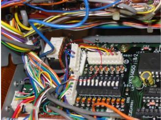
**Photo 8**: View of the back of the TS440 front face which was rocked. The PB "Voice" is connected to the "Control Unit" board by the J54 connector, which should be dismounted. This connector is very
