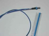
**Photo 7**: Preparation of two-wire connector between the command board of the DSP and the PB "Voice". The connector is made with from a standard Harwin style 0.1" pitch pin header. The wire colours, purple and blue, were chosen to conserve the colours used in the J54 connector, which arrives on the "Control Unit" board.
