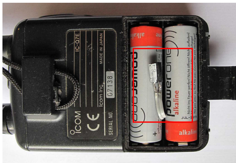
Photo 6: The wires emerge between the 2 batteries that are separated by an interval of 1 mm. The connector is folded between the batteries. The compact shaped connector does not interfere with the battery cover.
