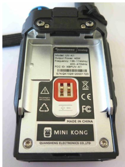
Photo 3: To open the UV-K1, remove the two Torx screws in the lower part, then lift the board along with its shielding.
