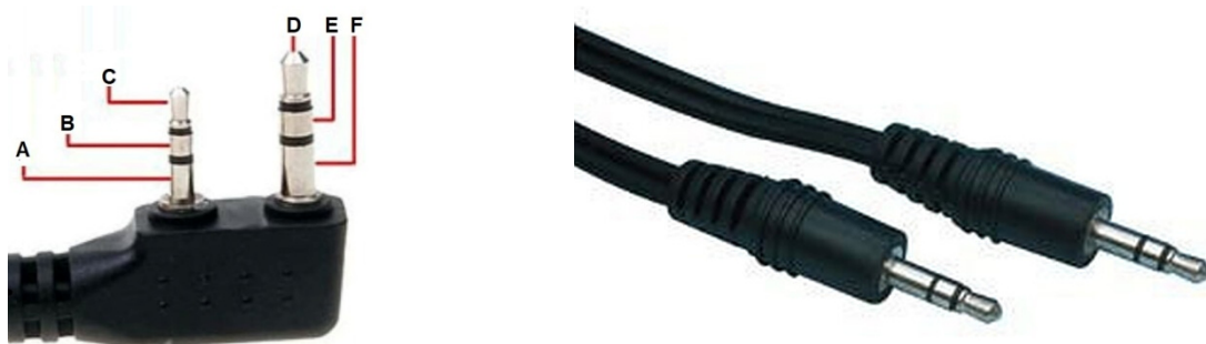
Photo 10: On the UV-K1's K-type connector, the output is on the tip (D) and the virtual ground is on the ring (E). A simple 3.5 mm jack cable is all that's needed to connect the UV-K1 to the decoder (Credit Photo A F6GVH).
